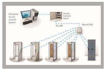
A featured solution available from ASSA ABLOY Group brands Corbin Russwin and SARGENT is the IN100 lock with Aperio® Technology offering remote lock/unlock in less than 10 seconds, streamlined design with choice of black or white reader, 50+ levers and 14 finishes, simultaneous support for HID Mobile Access® and multiple credential types including smart cards and Prox.
